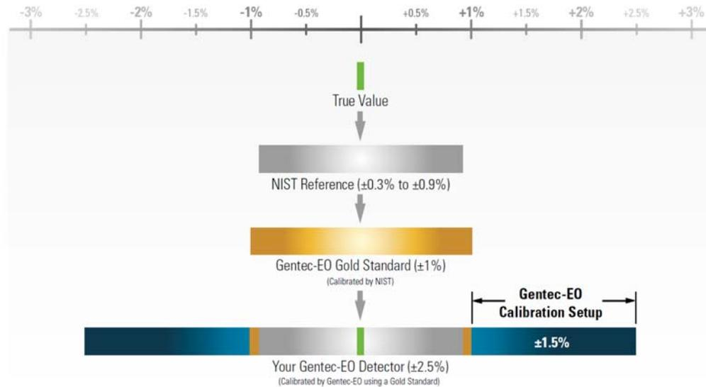
Before we perform the calibration measurements, the detector under test is allowed to reach equilibrium with the laboratory environment. The instrument’s sensitivity is found by dividing the instrument output reading by the incident laser power, which is measured by a traceable standard.
