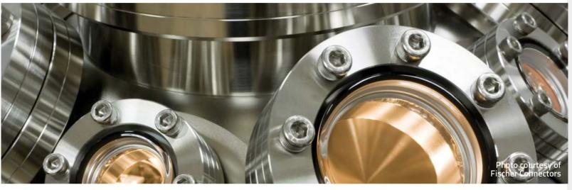
Depending on the experiment requirements, different degrees of vacuum can be obtained. The quality of a vacuum is determined by the amount of matter remaining in the environment and can therefore be measured by the total pressure. Ultra high vacuums can reach pressures as low as 10<sup>-9</sup> Pa and involve experimental challenges that one has to consider in order to design an experimental setup.
