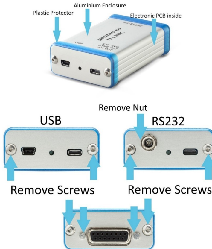
Figure 7. Opening U-LINK for recycling disposal
