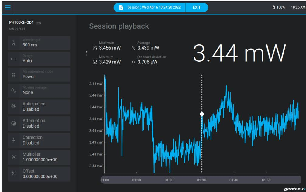
When the recording time is longer than the available time range, you can slide your finger on the time range to scroll through the data. To exit the recording viewer, tap on **Exit** in the upper part of the screen and confirm you want to exit the session playback.
