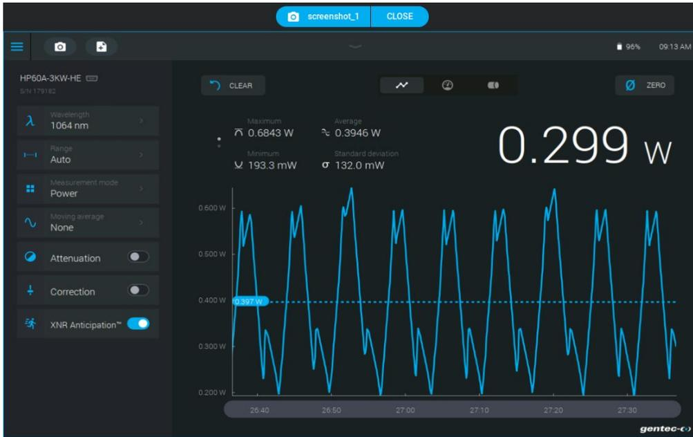
When viewing a recording, the detector settings will be shown in the left panel. These settings are also written in a human-readable format in the .txt file log when the log file is opened in a text editor on a PC.
