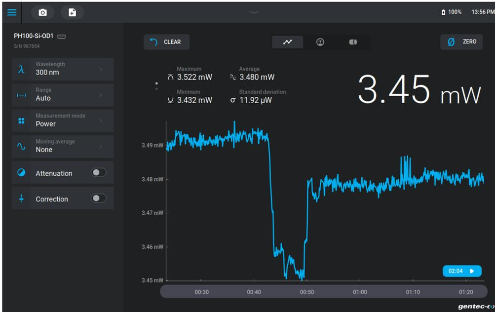
In the scope display, you may control whether the average cursor is visible or not. Press on the graph area for 1 second to activate or deactivate the average cursor. When the average cursor is activated in the scope display, it is also visible in the needle and bar displays.
