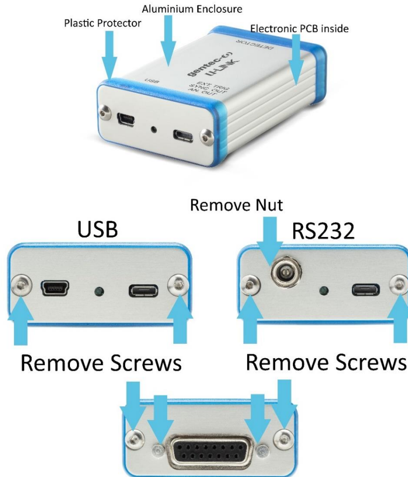
Figure 7 Opening U-LINK for Recycling Disposal
