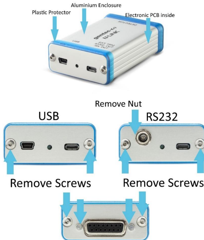
Figure 7. Opening U-LINK for recycling disposal
