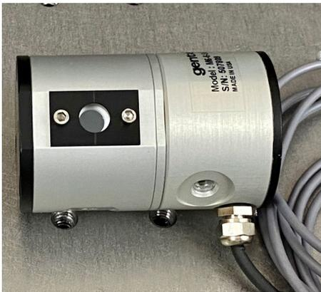
The standard M6-6-Si Joulemeter probe, shown here, includes a small 1 inch integrating sphere attached to the silicon detector cylindrical housing.
