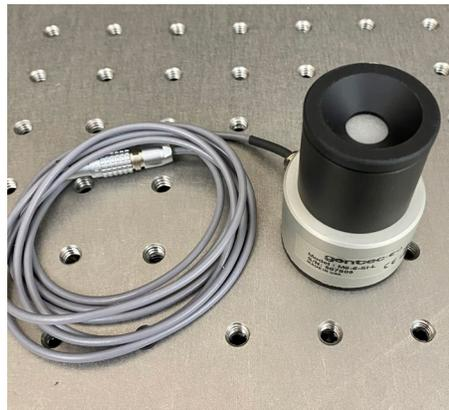
To attach the M6-UV-QED to the M6-6-Si probe, start by unscrewing the integrating sphere body from the detector body. They are held together by an SM1 thread. Then thread the M6-UV-QED diffuser into the detector body.
