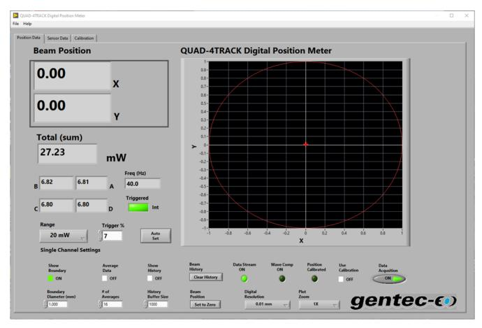
The Measurement Display has Controls and Indicators related to instrument usage. It is the main display used while taking data with the QUAD-4TRACK Instrument.
