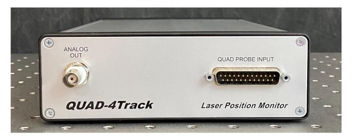
Figure 1, QUAD-4TRACK Front Panel
