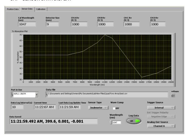
The Sensor Data Display has Controls and Indicators related to the sensor. The sensor information is read from the sensor memory on program startup.
