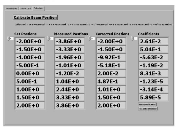
The Calibration Display has Controls and Indicators related to calibrating the beam position.
