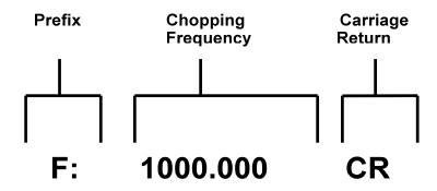
To set the chopping rate to 1 KHz on the high speed range, send the following eleven character string:
