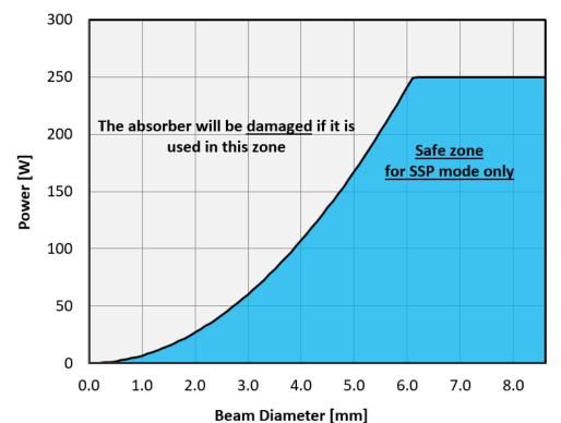
Figure 2 Minimum Beam Size for PRONTO-250 and PRONTO-250-PLUS absorber at 1064 nm in SSP mode
