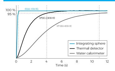
Inherently faster than thermal detectors and water calorimeters thanks to their photodiode-based sensor, integrating spheres of the IS series allow average powers of up to 1 kW to be measured in under 200 ms, tens of times faster than with both other technologies. This gives users the opportunity to follow the ramp-up of high-power sources and to discern relatively quick changes in laser power.
