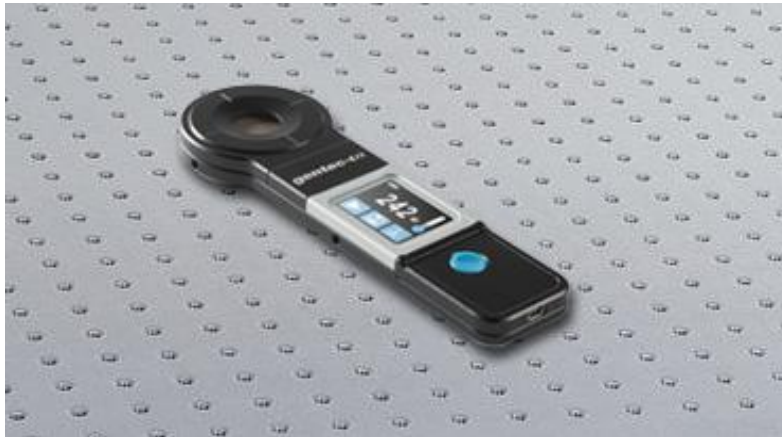
Figure 9. Recommended setup when making a measurement: install the device flat on a horizontal surface and illuminate from above
